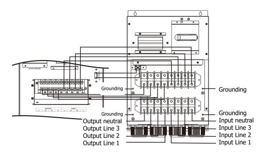
**NOTE:** Make sure that the wires are connected tightly with the terminals. Put the terminal block cover back to the rear panel.
